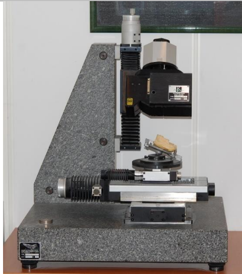
Figure 2: CICERO®: First laser-line laboratory scanner [12].
